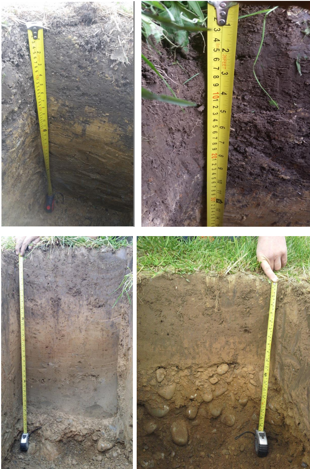
Figure 4. Upper : Southland . Left typical soil profile, depth 70 cm. Right: upper topsoil to 30 cm Lower: Canterbury. Left: deep phase, gravel depth 64 cm. Right: shallow, gravel 30 cm.
